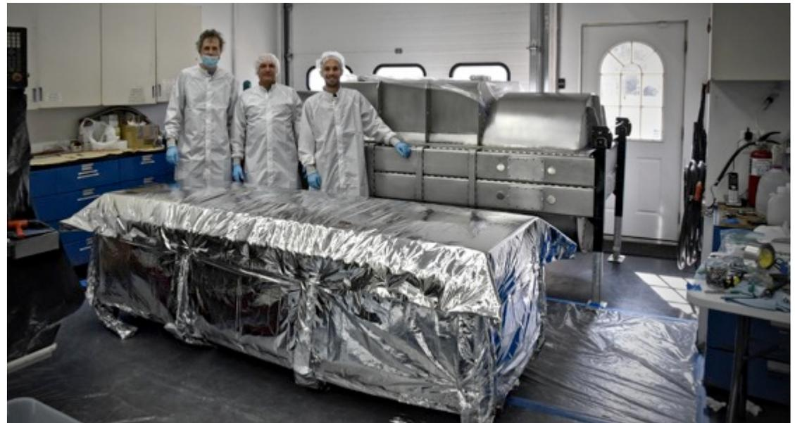
The HPF and NEID have demonstrated long-term stable control at the 1mK temperature level and  $<10^{-6}$  Torr pressure level
